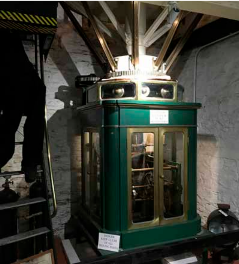
The images on this page add context to the Fresnel designs just discussed. All photos taken in the Wick Museum, Scotland. ABOVE LEFT: A perfect example of the base of the Fresnel design on the opposite page is shown here. The entire weight of the optical machinery rests on a base with rollers that are driven by a clockwork motor. ABOVE RIGHT: At the bottom of the optic is a group of prisms surmounted by the bull's eye arrangements. At the top are the mirrors designed by Fresnel. BELOW: Before electricity, multi-wick burners were at the focal point. Note venting was necessary for heat and gases to escape.
