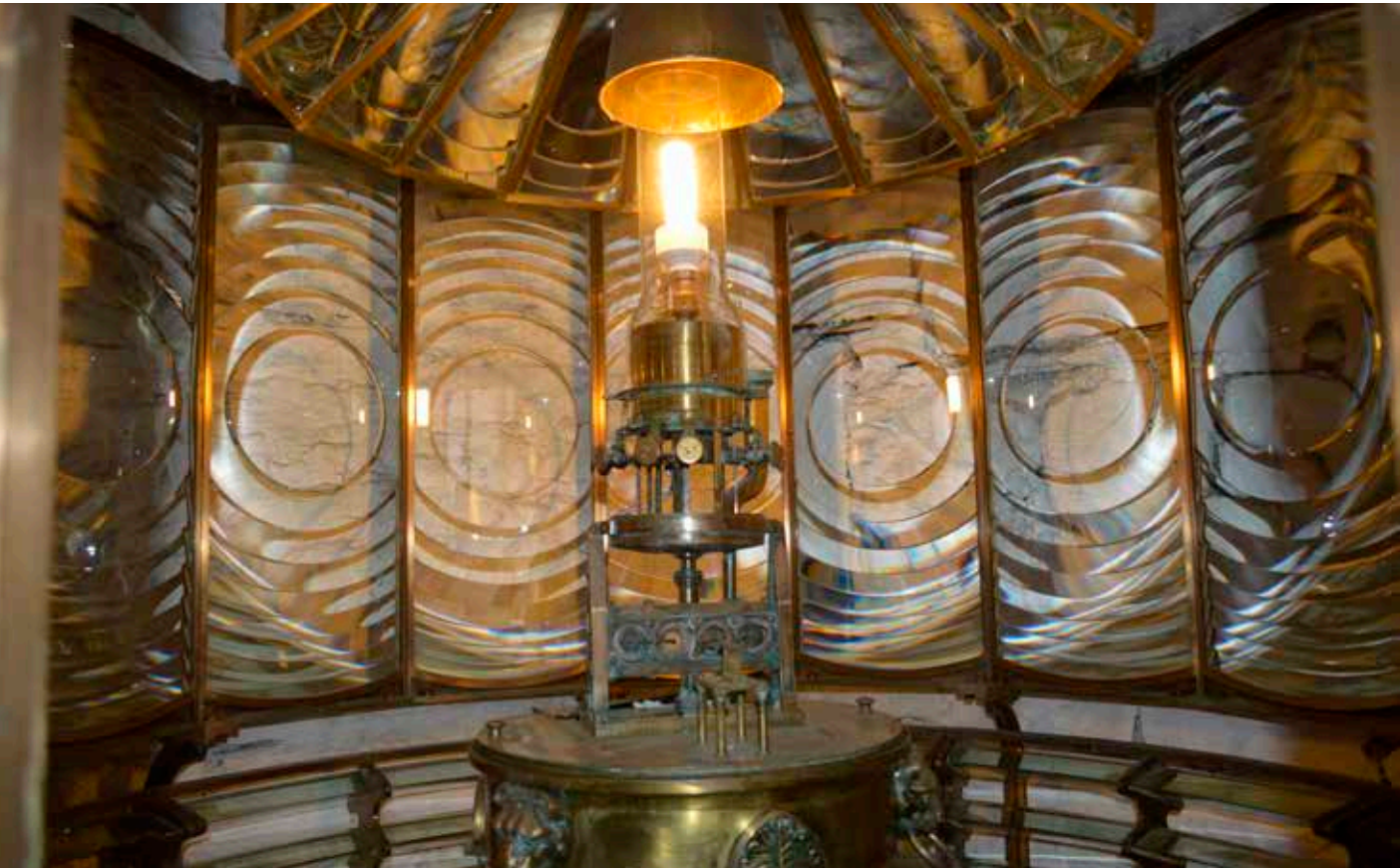
The images on this page add context to the Fresnel designs just discussed. All photos taken in the Wick Museum, Scotland. ABOVE LEFT: A perfect example of the base of the Fresnel design on the opposite page is shown here. The entire weight of the optical machinery rests on a base with rollers that are driven by a clockwork motor. ABOVE RIGHT: At the bottom of the optic is a group of prisms surmounted by the bull's eye arrangements. At the top are the mirrors designed by Fresnel. BELOW: Before electricity, multi-wick burners were at the focal point. Note venting was necessary for heat and gases to escape.
