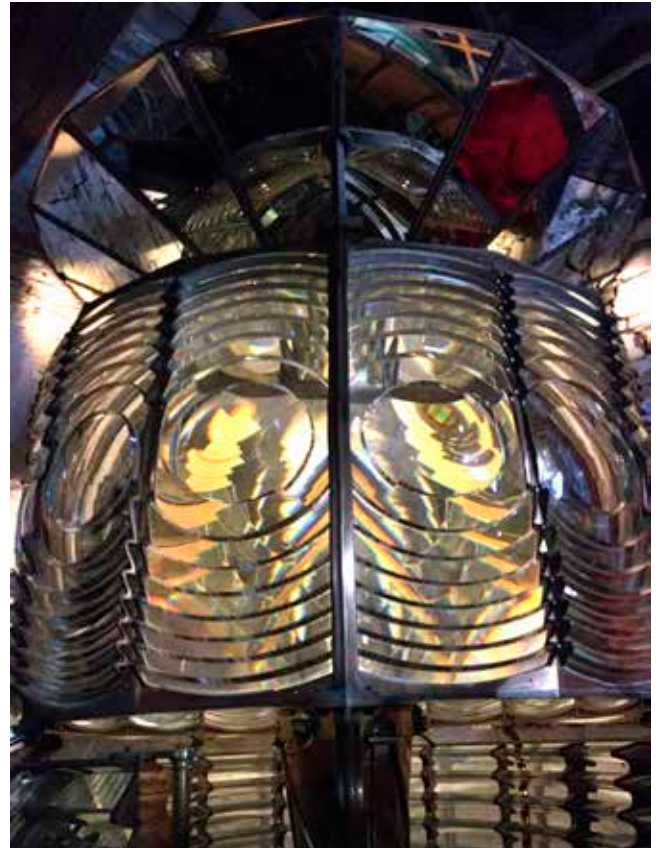
The images on this page add context to the Fresnel designs just discussed. All photos taken in the Wick Museum, Scotland. ABOVE LEFT: A perfect example of the base of the Fresnel design on the opposite page is shown here. The entire weight of the optical machinery rests on a base with rollers that are driven by a clockwork motor. ABOVE RIGHT: At the bottom of the optic is a group of prisms surmounted by the bull's eye arrangements. At the top are the mirrors designed by Fresnel. BELOW: Before electricity, multi-wick burners were at the focal point. Note venting was necessary for heat and gases to escape.
